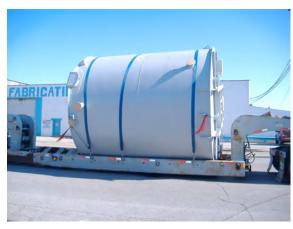
For tanks that are constructed at the plant (rather than in the field), fabrication entails sophisticated processes and equipment plus the availability of metals containing specific alloys. Fabrication facilities must include extensive lifting capabilities and equipment such as heavyduty break presses, plate rolls, automated submerged-arc welding, and CNC plasma burning machines.
